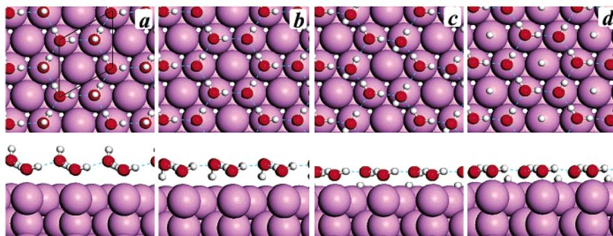
**Figure 3.** Top and side views of (a) “H-up” intact bilayer, (b) “H-down” intact bilayer, (c) the transition state for bilayer dissociation, and (d) the partially dissociated OH–H<sub>2</sub>O+H overlayer. The parallelogram in (a) indicates the surface,  $(\sqrt{3} \times \sqrt{3})R30^\circ$  unit cell.
