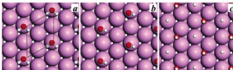
**Figure 1.** Structures of the initial (a), transition (b), and final states (c), of H<sub>2</sub>O monomer dissociation on Ru{0001}. The parallelogram in (a) indicates the surface, p(2 × 2), unit cell.
