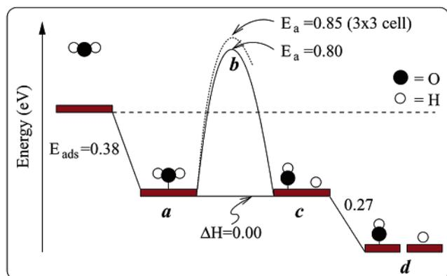
**Figure 2.** Relative energy diagram for H<sub>2</sub>O monomer adsorption and dissociation on Ru{0001}. The states labeled a, b, and c correspond to the structures shown in figure 1a, 1b, and 1c, respectively. State d corresponds to OH and H chemisorbed in separate unit cells. All energies, unless indicated otherwise, are for a p(2 × 2) unit cell.
