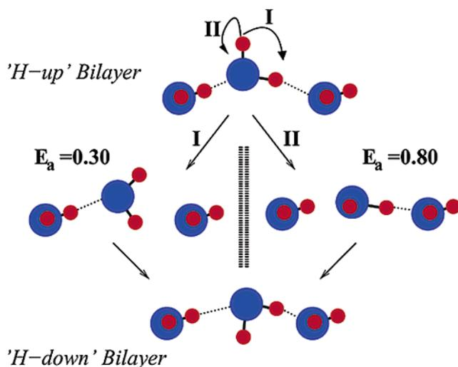
**Figure 4.** A schematic diagram (side view) illustrating the two mechanisms investigated for the conversion of a “H-up” into a “H-down” intact bilayer on Ru{0001}. For clarity, the Ru surface is not shown.
