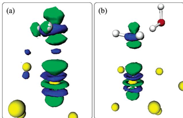
**Figure 8.** Isosurfaces of the difference electron density upon adsorption for (a) H<sub>2</sub>O monomer adsorption and (b) H-up intact bilayer adsorption. Blue contours indicate an electron density increase of  $3 \times 10^{-2} e/\text{\AA}^3$ ; green contours indicate an electron density decrease of  $3 \times 10^{-2} e/\text{\AA}^3$ .
