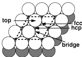
FIG. 1. Top view of the Ni(111) surface. The dashed lines represent the surface unit cell, the arrows indicate the position of the four high symmetry sites. For clarity, only two Ni layers are shown.
