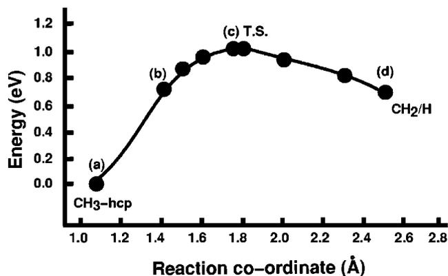
FIG. 4. Total energy in eV, relative to the initial state, for the lowest energy reaction pathway. The reaction coordinate in Å is the distance between carbon and the active hydrogen. (a), (b), (c), and (d) refer to the points shown in Fig. 3. The solid line is an aid to the eye.
