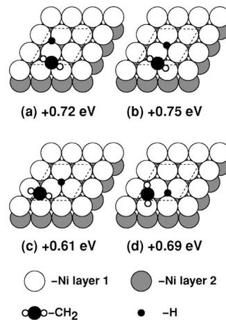
FIG. 2. The four CH<sub>2</sub>/H coadsorption arrangements identified within the  $p(2 \times 2)$  unit cell. The energies of these arrangements relative to CH<sub>3</sub> chemisorbed on an hcp site are also shown. The periodic nature of the systems are not shown for clarity.
