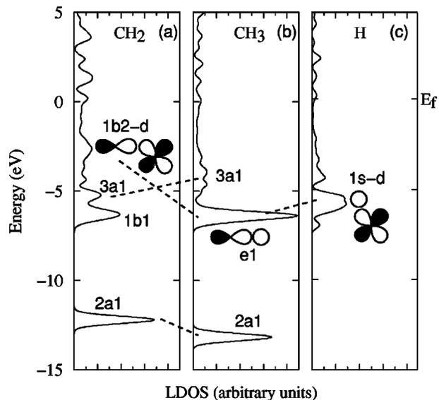
FIG. 5. Local densities of states plots (LDOS) for  $\text{CH}_2$ ,  $\text{CH}_3$ , and H at their preferred chemisorption sites on Ni(111). The Fermi levels ( $E_f$ ) of each system have been aligned to 0 eV. A partial energy level interaction diagram has been superimposed upon the plots highlighting the most significant orbital changes that occur upon going from  $\text{CH}_3(\text{ads})$  to  $\text{CH}_2(\text{ads}) + \text{H}(\text{ads})$ .
