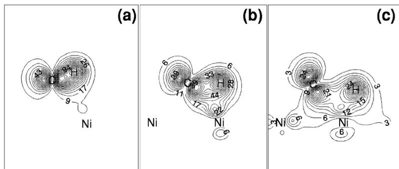
FIG. 6. 2D electron density contour plots for an  $e_1$  derived quantum state at certain points along the reaction pathway. The quantum states in (a), (b), and (c) are taken from the points (a), (b), and (c), in Fig. 3. The planes of the 2D cuts are through the C–H bond normal to the surface. Density is plotted in units of  $3.63 \times 10^{-3}$  electrons/bohr<sup>3</sup>.
