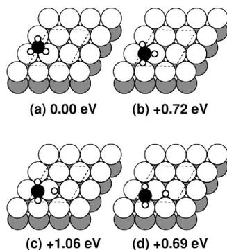
FIG. 3. The lowest energy reaction pathway identified for  $\text{CH}_3$  dehydrogenation on Ni(111). (c) is the transition state. For clarity, the periodic nature of the systems is not shown.
