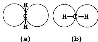
FIG. 4. Schematic structures of the two initial orientations of  $\text{CH}_2$  adsorbed at the bridge site. (a) C is in a tetrahedral environment. (b) C is in a planar environment.
