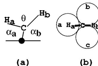
FIG. 3. Schematic structure of CH<sub>2</sub> adsorbed at a threefold hollow site.  $\alpha_a$  and  $\alpha_b$  are the surface-C-H<sub>a</sub> and surface-C-H<sub>b</sub> angles, respectively. (a) is viewed from the side. The horizontal line represents the center of the top layer of Ni atoms. The small black circle indicates the center of the threefold hollow site. (b) is viewed from above, the Ni surface is represented by circles.
