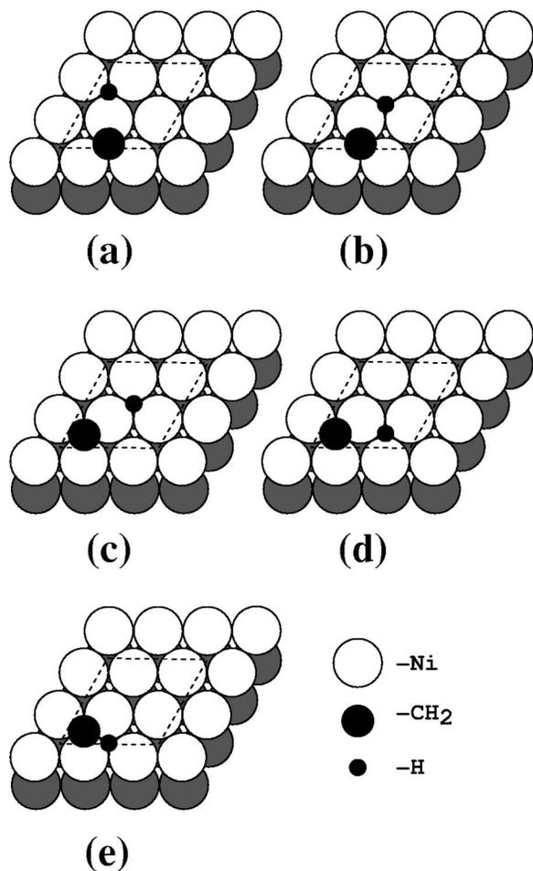
FIG. 8. The five  $\text{CH}_2/\text{H}$  coadsorption systems calculated. For clarity, the periodic nature of the systems is not shown.
