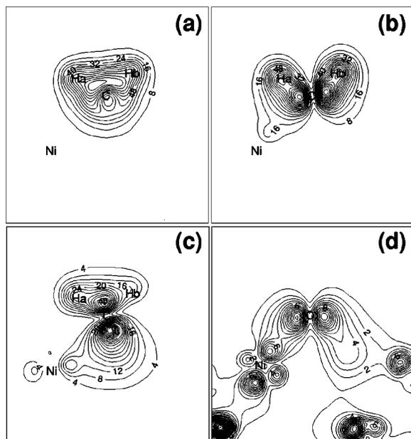
FIG. 7. 2D electron density contour plots of some typical quantum states for CH<sub>2</sub> adsorbed at the fcc threefold hollow site of Ni(111). The plane of the cuts (a)–(c) is through the C-H<sub>a</sub>-Ni<sub>a</sub> nuclei. The plane of slice (d) is orthogonal to that used in (a)–(c). Density is in units of  $3.63 \times 10^{-3}$  electrons/bohr<sup>3</sup>.
