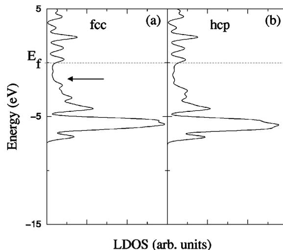
FIG. 2. Local density of states (LDOS) projected onto a 0.5 Å radius centered on H at the fcc and hcp sites. The Fermi levels have been aligned and set to 0 eV. The arrow indicates the center of the substrate density of states prior to adsorption.
