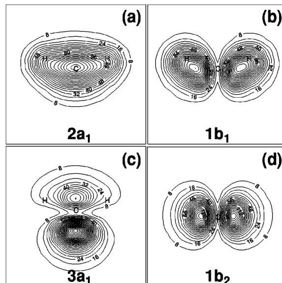
FIG. 5. Two-dimensional (2D) electron density contour plots for the four occupied orbitals of  $\text{CH}_2$  in  $^3B_1$ . The plane of the cuts (a)–(c) is through the C-H-H nuclei. The plane of slice (d) is orthogonal to that used in (a)–(c). Density is in units of  $3.63 \times 10^{-3}$  electrons/bohr $^3$ .
