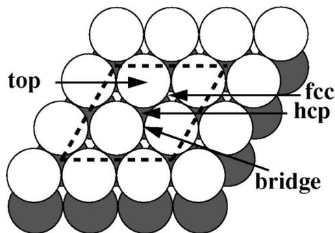
FIG. 1. A section of the Ni(111) surface. The arrows indicate the position of the four high symmetry adsorption sites. The dashed line represents the unit cell. Only two layers of metal atoms are shown for clarity.
