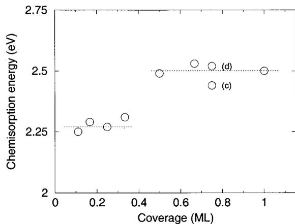
FIG. 1. Coverage dependence of OH chemisorption energy on Pt(111). At 0.75 ML two values (c and d) are given, corresponding to two different overlayers, shown in Figs. 3(c) and 3(d), considered at this coverage.
