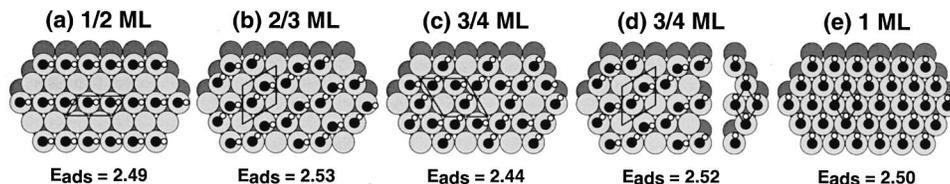
FIG. 3. Plan views of the most stable high coverage (1/2 ML  $\rightarrow$  1 ML) pure OH phases on Pt(111). (d) illustrates how 3/4 ML OH can be partitioned into majority  $\sqrt{3} \times \sqrt{3} - R30^\circ$  (76%) and minority  $(1 \times 1)$  (24%) domains.
