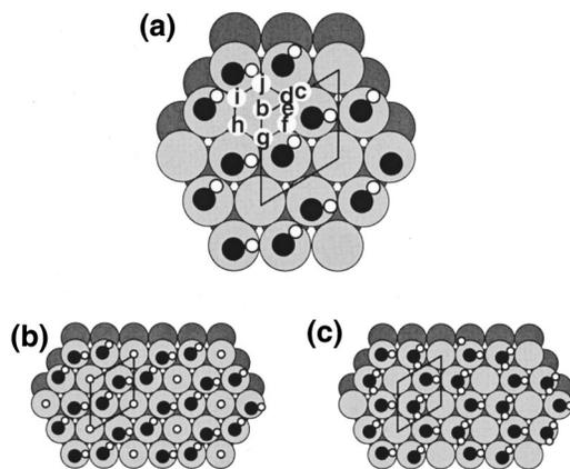
FIG. 4. (a) OH+H coadsorption systems with  $b$ - $j$  being the possible H positions considered. (b) and (c) are the two types of optimized structure obtained from the nine initial coadsorption systems. (b) is an OH+H coadsorbed phase. (c) is a mixed OH+H<sub>2</sub>O phase.
