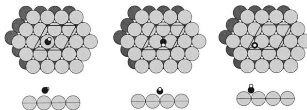
FIG. 2. Low coverage structures of OH adsorbed at the top, bridge, and fcc sites of Pt(111). Gray, black, and white circles correspond to Pt, O, and H atoms, respectively. Only two surface layers are shown for clarity. The solid lines represent the surface unit cell.
