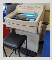
A chilled microtome for the cutting of frozen sections of 1-100 microns in thickness at temperatures down to -30°C. It has a quick freeze function for rapid cooling of samples and a UVC disinfection to maintain sample sterility.
