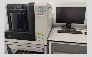
A high-throughput brightfield digital scanner that can handle batches of up to 360 slides at a time to produce digital images in the .ndpi format at either 20x or 40x resolution. Capable of scanning speeds of 1 slide in 30s (at 20× mode for a 15 x 15mm area). Incorporates slide label anonymisation at point of scanning
