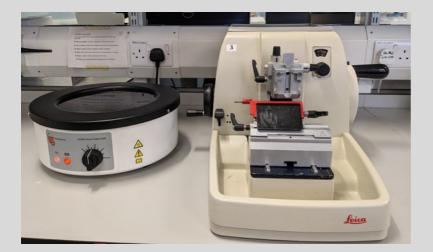
We have 3 manual rotary microtomes available for the precision cutting of tissue sections between 1-60 microns in thickness as well as waterbaths for floating out sections
