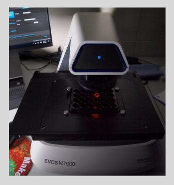
The Evos M7000 is a multipurpose widefield based imaging system. It is equipped with a colour camera to image coloured stains as well as a monochrome camera for fluorescence imaging.
