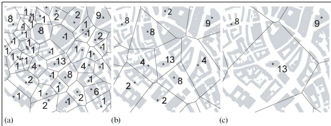
Figure 6: Landmarks and dominance regions (Voronoi partitions) with different levels of detail: a) base level; b) level 1; c) level 2 (Winter et al. 2008, 390)
