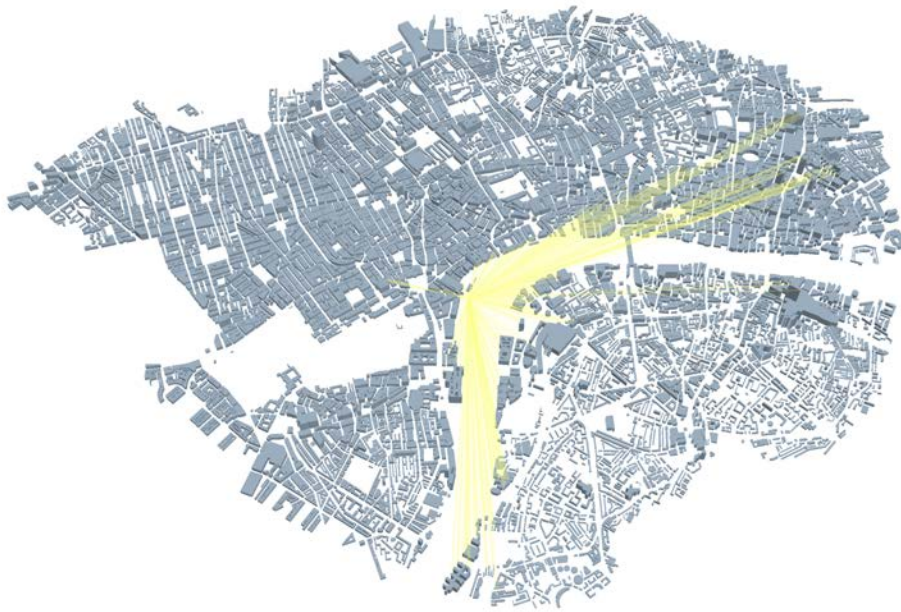
Figure 9: Visible sight lines from an observer point in ArcScene, Congestion Charge Zone, London.
