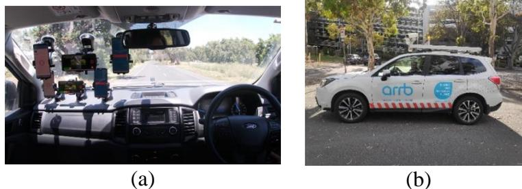
Figure 1 (a) the in-cabin set up and (b) the ground-truth survey vehicle
