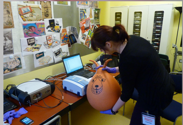
Fig 2. Using infrared spectroscopy to identify plastics in the Museum of Childhood.
