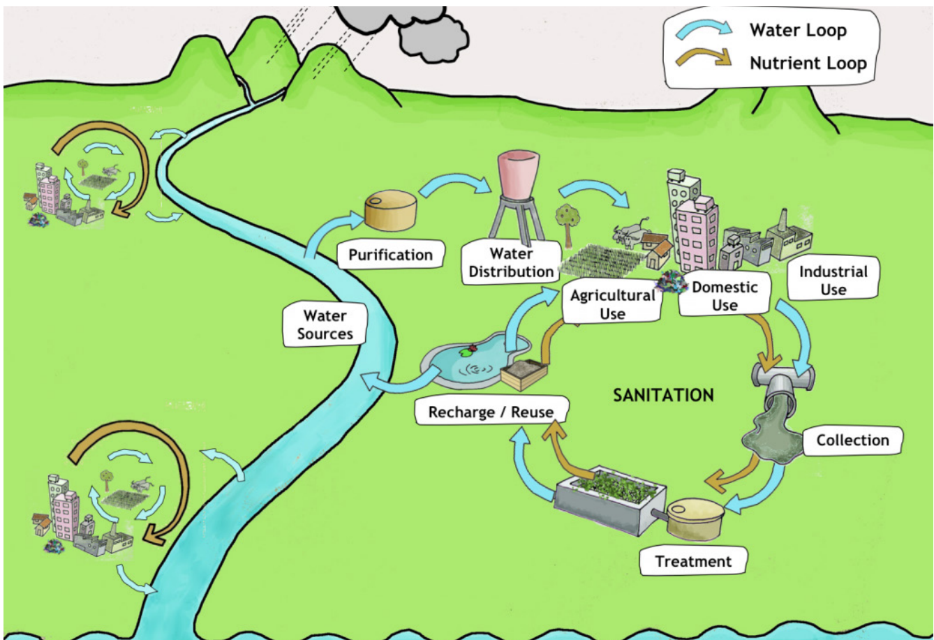
Figure 2.4. Simplified water and nutrient loops. Source: Conradin (2013)
