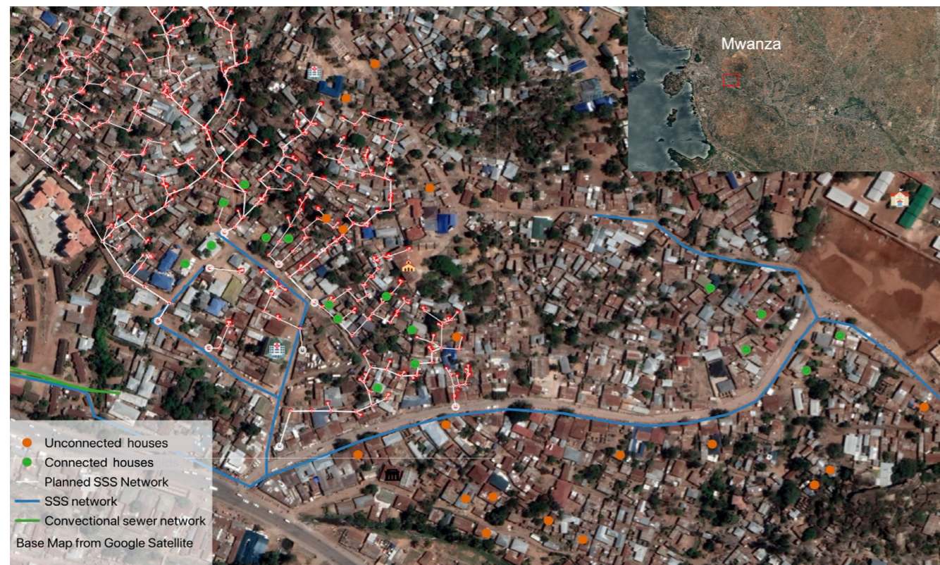
Figure 2: Map of sanitation connections and houses visited during fieldwork conducted in April-May 2023. Mabatini settlement, Mwanza, 2023. Source: Authors.
