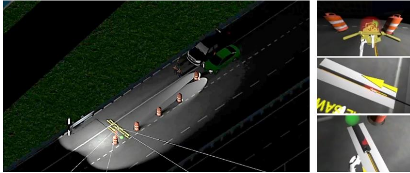
Figure 3: Virtual model overview (left) and example user interactive tasks in VR (right) for short-term highway work zone for installing PVDF sensor.
