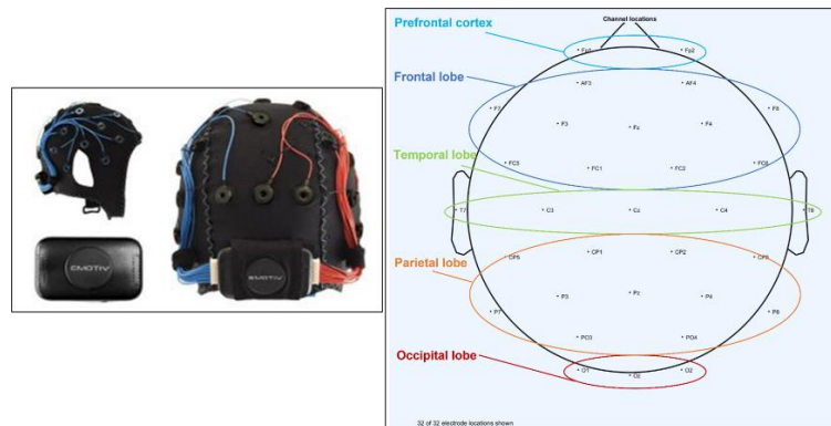
Figure 2: EEG headset for data collection and 32 channels in different brain regions
