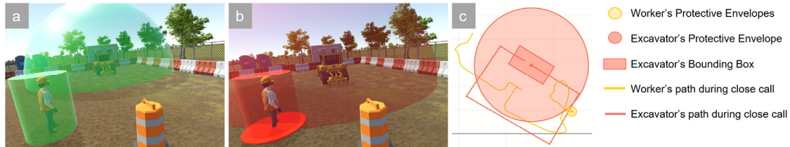
Figure 3: (a) Dozer representing hazard, (b) a collision of the safety envelopes, and (c) the recorded trajectory data related to the close call.
