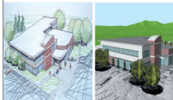
Figure 3 The original architectural drawing of a modern office building (left) and the same building rendered in a 3D GIS display (right) with the surrounding terrain from a digital elevation model in the background. Note that the look and white architectural style has been retained, updated, and draped over the terrain model. Unlike the drawing, the 3D presentation can be viewed from any location in the scene.
