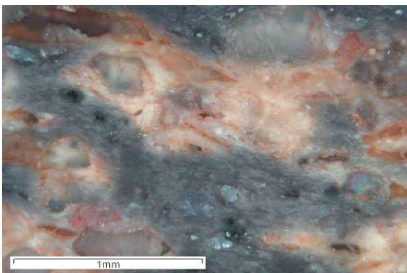
Figure 2 A cross-section of the fabric of a Hessian crucible found in Cripplegate, London (WFG 18/129/s2), under cross-polarized light ( \times 50 ), showing the characteristic appearance of unused Hessian crucibles; that is, alternating grey and orange areas. A few spheroidal iron-rich minerals (dark) and molten feldspars are the only notable inclusions in addition to the quartz temper.
