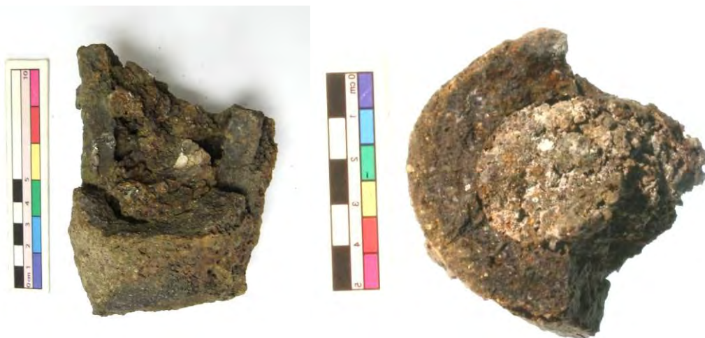
Figure 5.20 Left: rusty slag with white inclusions in SDB7; right: top view of slag in SDB12.
