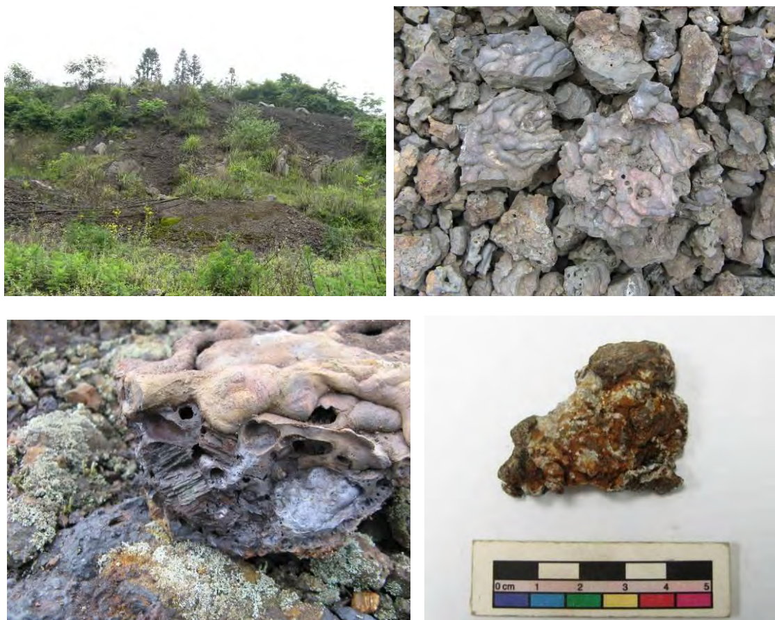
Figure 5.4 Top left: slag heaps from the Laochangping site; top right: tap slag with clear flowing structures from the Laochangping site; bottom left: charcoal trapped inside the slag from the Luzhadui site; bottom right: a lead fragment from the Laochangping site.
