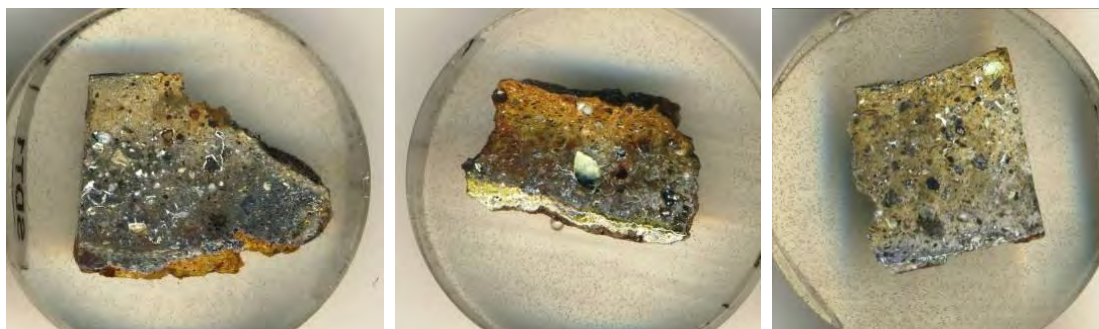
Figure 5.16 Cross sections of condenser SDT1 (left), SDT2 (middle) and SDT3 (right). The internal surfaces of these samples are facing up.
