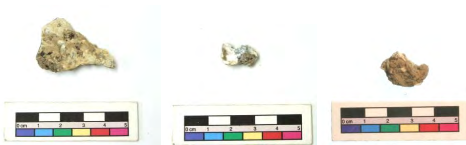
Figure 4.19 Three lumps of zinc metal from Miaobeihou: YMZ1 (left), YMZ2 (middle) and YMZ3 (right).
