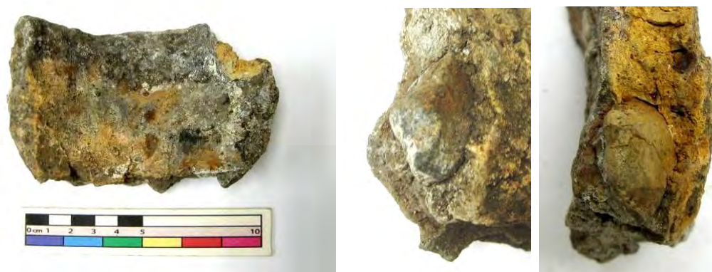
Figure 5.15 Left: the internal surface of SDT1; middle: a large inclusion in SDT3; right: a large inclusion in SDT5.
