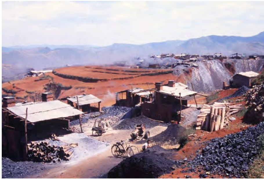
Figure 4.77 A traditional zinc smelting workshop at Ya Kou near Zhehai, Yunnan province (photo by Paul T. Craddock, May 1995). The two sheltered saddle furnaces in the front were surrounded by piles of retorts, coal and possible ores/mixed charge. The machine in the middle was used for mixing ores and coal.
