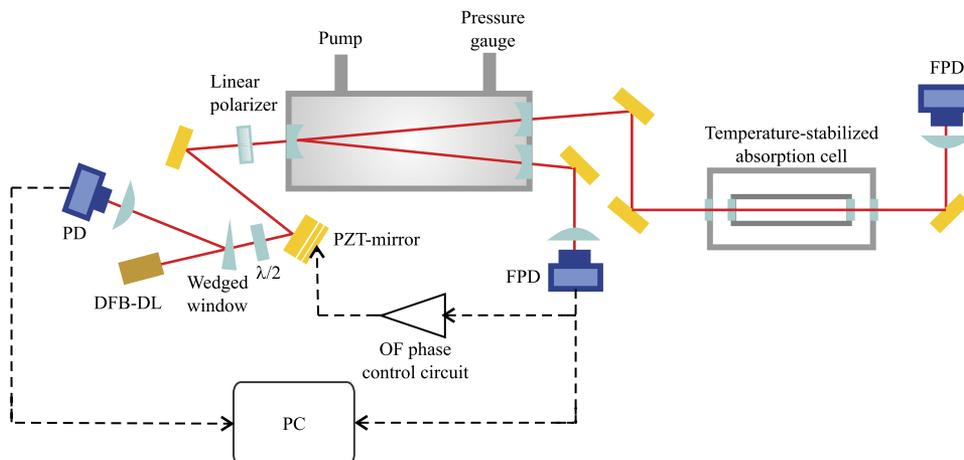
FIG. 1. Sketch of the laser absorption spectrometer. DFB-DL stands for distributed-feedback diode laser, PD for photodetector, FPD for fast photodetector, PZT for piezoelectric actuator, and  $\lambda/2$  for half wave plate.
