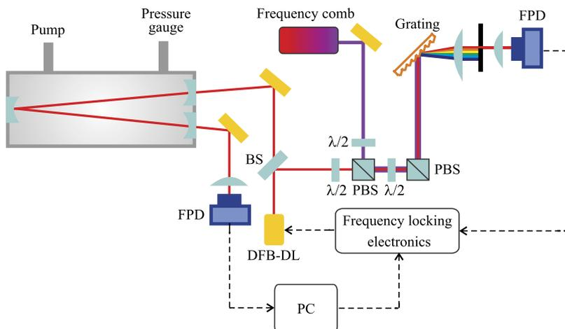
FIG. 3. Sketch of the setup for cavity FSR measurements. DFB-DL - distributed-feedback diode laser, FPD - fast photodetector, BS - beam splitter, PBS - polarizing beam splitter,  $\lambda/2$  - half wave plate.
