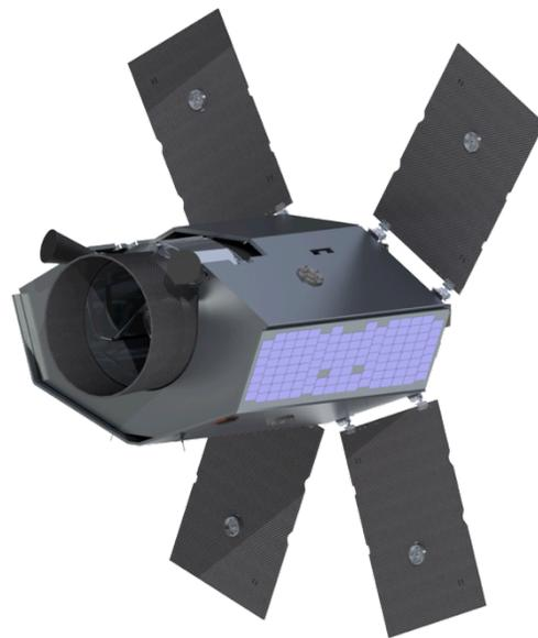
*Figure 1: A representation of the Twinkle satellite, based on an SSTL-300 platform.*
