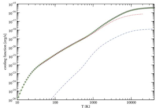
**Figure 1.** HD radiative cooling function. Circles: dipole contribution, present calculation; blue dot-dashed curve: quadrupole contribution; red dashed curve: high-density limit fit by Lipovka et al. (2005); green solid curve: fit given in Table 1.
