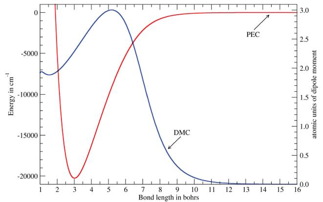
**Figure 6.** LiH potential energy curve (PEC) and dipole moment curve (DMC). The two curves use different scales for the y-axis; the left-hand side legend refers to the PEC and the right-hand side one to the DMC.
