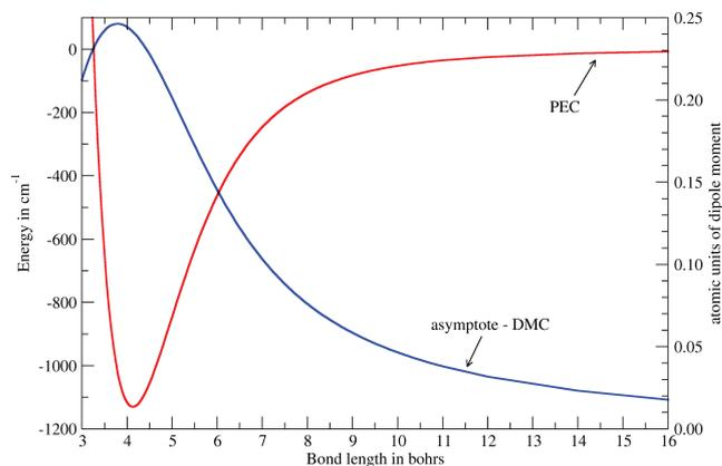
**Figure 8.**  $\text{LiH}^+$  PEC and the quantity  $0.125613r - M(r)$  (see text for details). The two curves use different scales for the y-axis; the left-hand side legend refers to the PEC, the right-hand side one to the DMC.
