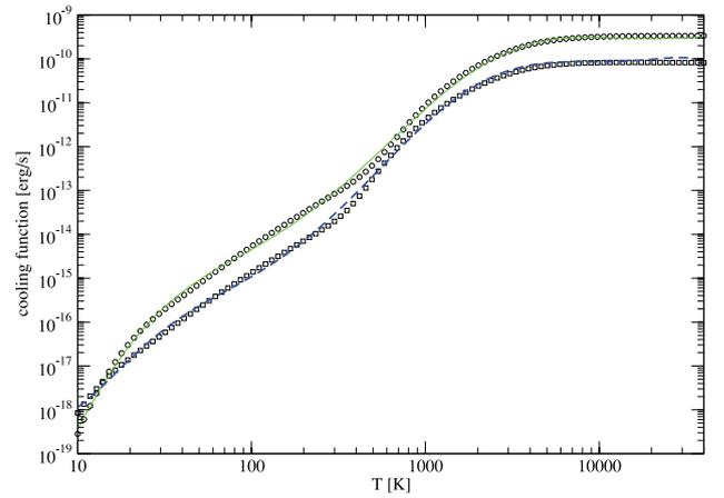
**Figure 4.**  $\text{HeH}^+$  radiative cooling function contributions. Circles:  $^4\text{HeH}^+$ ; squares:  $^4\text{HeD}^+$ ; green solid curve:  $^4\text{HeH}^+$  fit (Table 1); blue dashed curve:  $^4\text{HeD}^+$  fit (Table 1).
