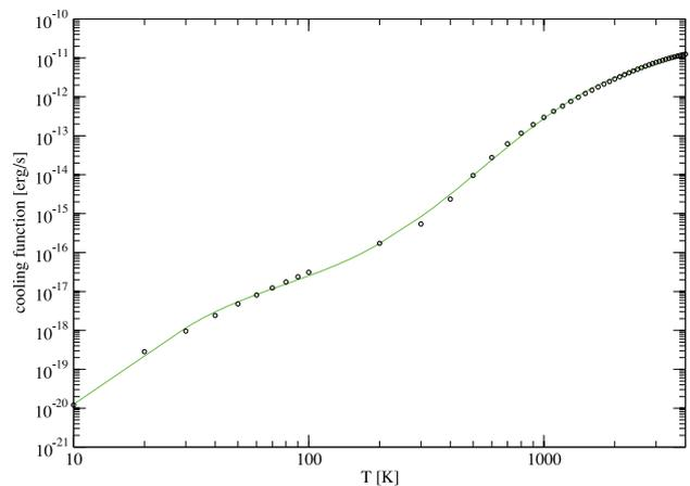
**Figure 9.** H<sub>2</sub>D<sup>+</sup> radiative cooling function. Circles: calculation by Sochi & Tennyson (2010); green solid line: fit given in Table 1.
