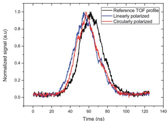
**Fig. 6** Time-of-flight (TOF) spectra of CS<sub>2</sub> in the molecular beam when perturbed by a linearly and circularly polarized field as well as the unperturbed reference TOF when the field is turned off.
