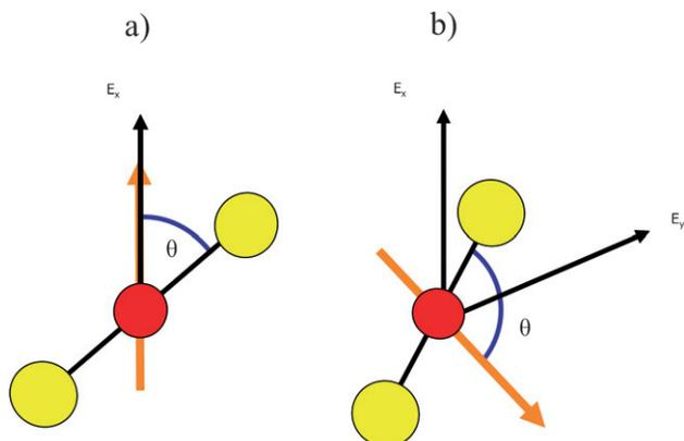
**Fig. 4** The orientation of the linear molecule  $\text{CS}_2$  with respect to the polarization vector for linearly and circularly polarized light defined by the angle  $\theta$ .
