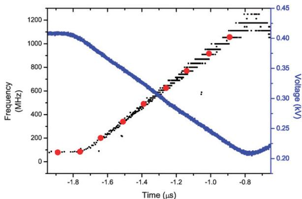
**Fig. 9** Frequency of the microchip laser measured as a function of time by heterodyning a fixed frequency laser demonstrating the greater than  $1 \text{ GHz } \mu\text{s}^{-1}$  frequency chirp required for deceleration experiments.
