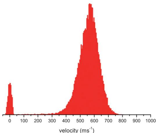
**Fig. 7** Simulated velocity distribution function after chirped deceleration of H<sub>2</sub> seeded into a molecular beam with an initial temperature of Ar at 560 K with a FWHM energy spread of 70 mK. The laser is chirped over 1.1 GHz in 150 ns and requires an energy of 60 mJ per lattice beam.
