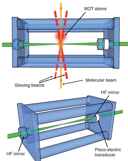
**Fig. 3** Fused-silica cavity design. Molecular slowing beams are shown in red, intersecting at the beam waist of the 532 nm (green) dipole trap beam at the centre of the cavity (the trapping point).
