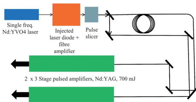
**Fig. 8** Schematic diagram of the chirped optical Stark deceleration system which amplifies the output from a Nd:YVO<sub>4</sub> laser up to 700 mJ in each arm over a 1  $\mu$ s interval.
