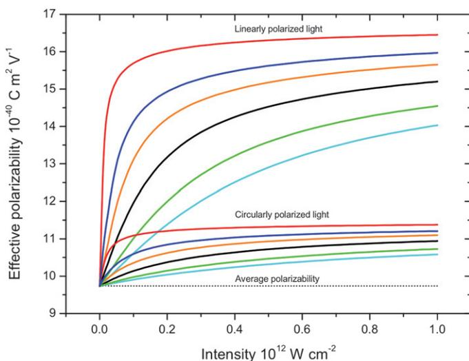
**Fig. 5** The effective polarizability is plotted against the nonresonant laser intensity for rotational temperatures 2 K (red), 4 K (dark blue), 6 K (orange), 8 K (black), 10 K (green), 12 K (light blue), for linearly polarized light and circularly polarized light. The average polarizability is also shown for comparison (dashed line).
