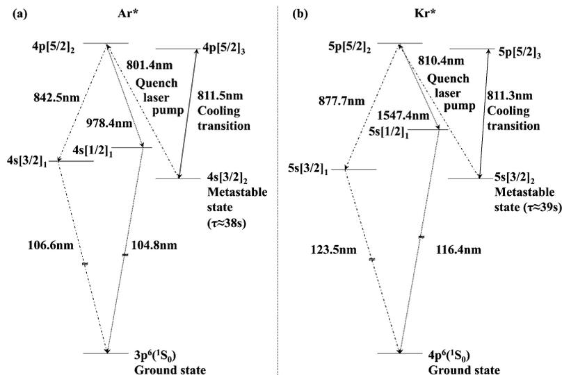
Fig. 1 Energy levels relevant for laser cooling and quenching of Ar\* and Kr\*.
