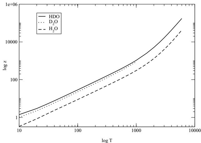
**Figure 1.** Comparison of HDO and D<sub>2</sub>O internal partition functions,  $z$ , as a function of temperature,  $T$ , computed in this work with the H<sub>2</sub>O partition function of Vidler & Tennyson (2000).
