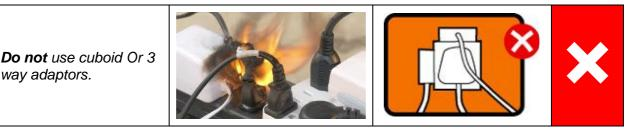
Only use 4 to 6 Way Gang Individually Switched UK<br/>fused Mains Extension Lead with a length of flex. The<br/>Maximum load for any one socket should not exceed 13<br/>amps.
