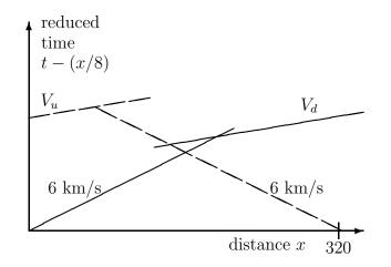
Solid lines: shooting down dip from a source at x = 0Dashed lines: shooting up dip from a source at x = 320 km
