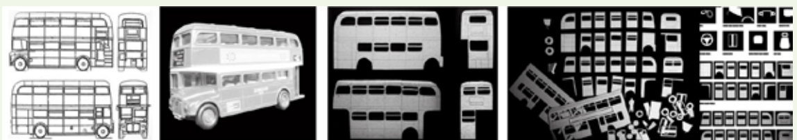
Figure 2: Clarification of Routemaster parts for their future reuse as the key building material
