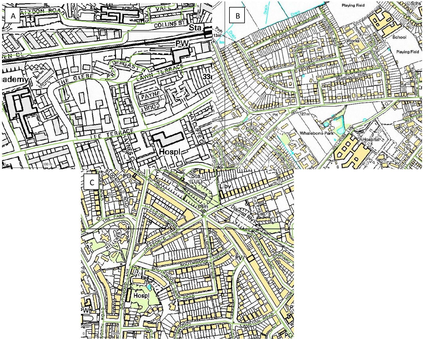
Figure 3 – Examples of overlapping OSM and OS maps for New Cross (A), Barnet (B) and Highgate (C). The green lines which overlay the map are OSM features.
