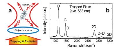
**Figure 2.** (a) Sketch of the Raman Tweezers setup. Trapping and excitation is performed with the same laser beam at 633nm. Collection of the Raman signal is guided through the same objective used for trapping. (b) Typical Raman spectrum for single layered graphene in the optical trap.
