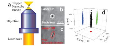
**Figure 1.** (a) Optical trapping geometry. (b) Image of a trapped nanotube bundle oriented by radiation torque along the optical axis. (c) Image of the same bundle un-trapped (laser is off) and randomly oriented by Brownian motion. (d) Tracking of a trapped nanotube bundle Brownian motion. The calibration of the trap allows force sensing with femtonewton resolution in liquid environment.
