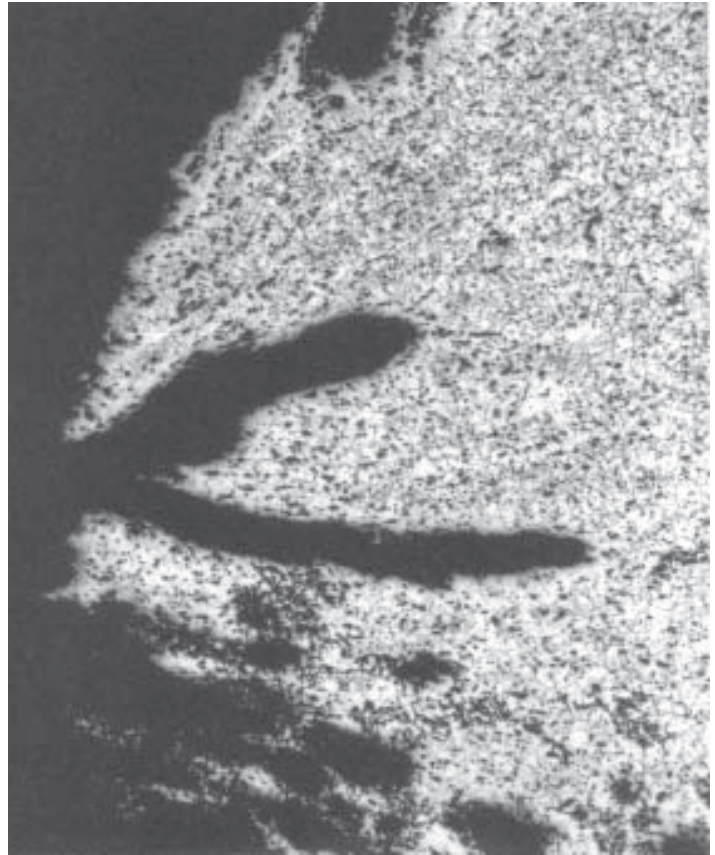
Fig. 2. Photomicrograph of the V-shaped fissure of cylindrical fragment. Note the flow of the deformed inclusions towards the edge. 50x mag. Etched; alcoholic ferric chloride.
