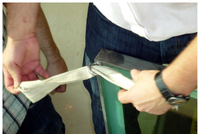
Guy threads lifting tapes through rings on the glass cover of the lightbox.
