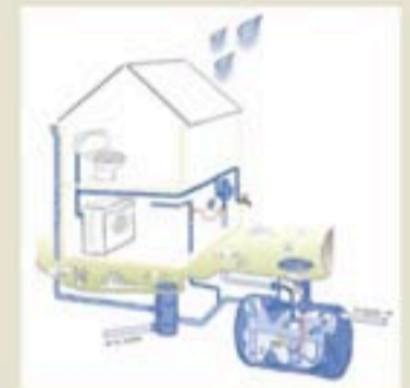
Caption 1: Schematic of a typical rainwater harvesting system (source: www.swiftps.com)
