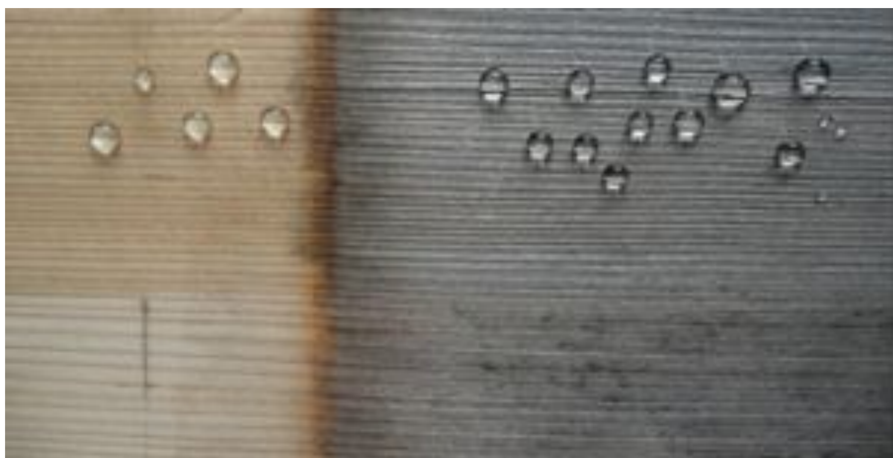
Figure 2: Effect of organofunctional silanes on surface hydrophobicity (Source: Empa)
