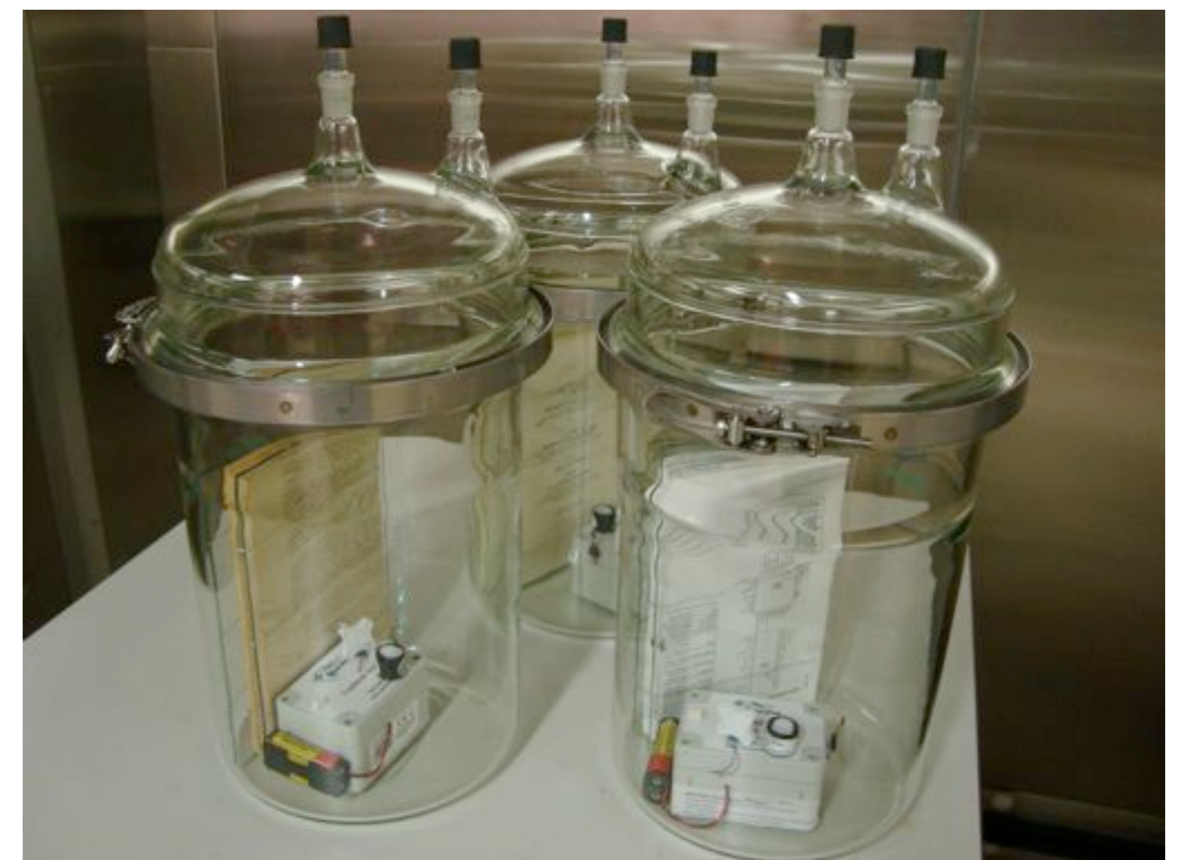
Measurement of emission and reabsorption of volatile compounds in porous materials (closed books).
