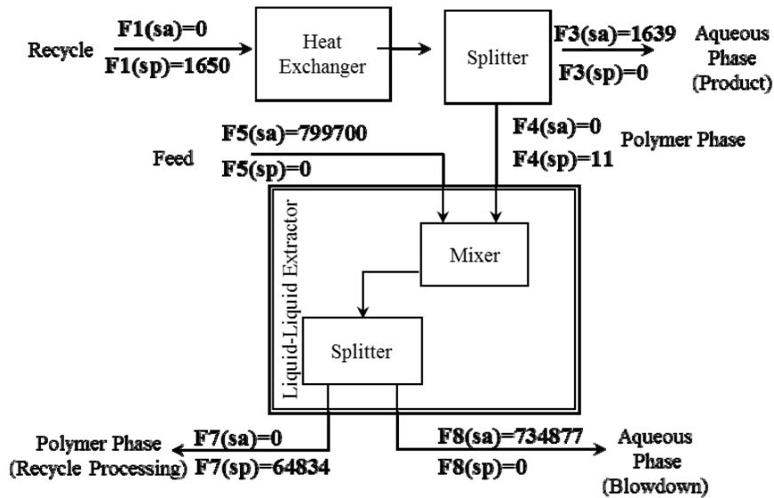
Figure 4. Salt flows for aqueous and polymer phase in lbs/hr
